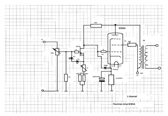
Therefore I applied the Vanderveen-Trans-circuitry: <u>http://www.elektor.com/vanderveen-trans-tube-amplifiers</u>. Please see the schematic below:
