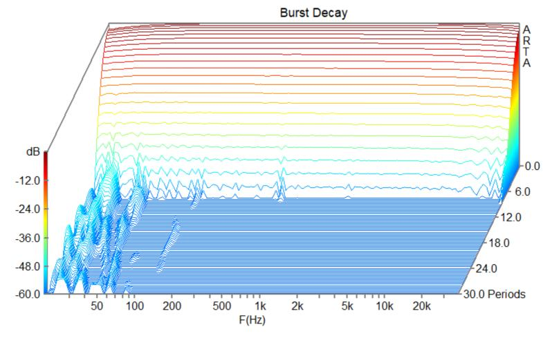
2024-05-18 Meting AMP Joop-300B-SE - BD 1W in 8 Ohm Right Channel
