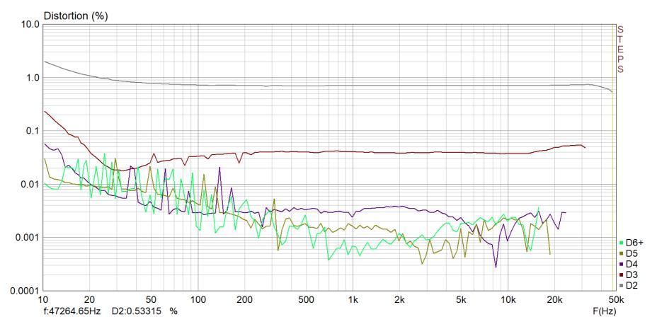
2024-05-18 Meting Joop-300B-SE - STEPS D% 1W in 8 Ohm Left Channel
