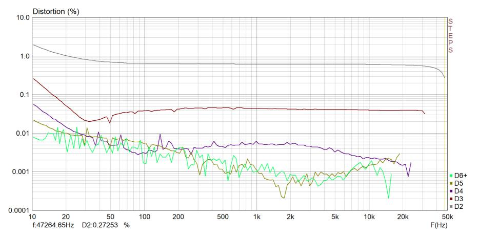
2024-05-18 Meting Joop-300B-SE - STEPS D% 1W in 8 Ohm Right Channel
