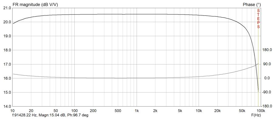
2024-05-18 Meting Joop-300B-SE - STEPS FR 1W in 8 Ohm Right Channel
