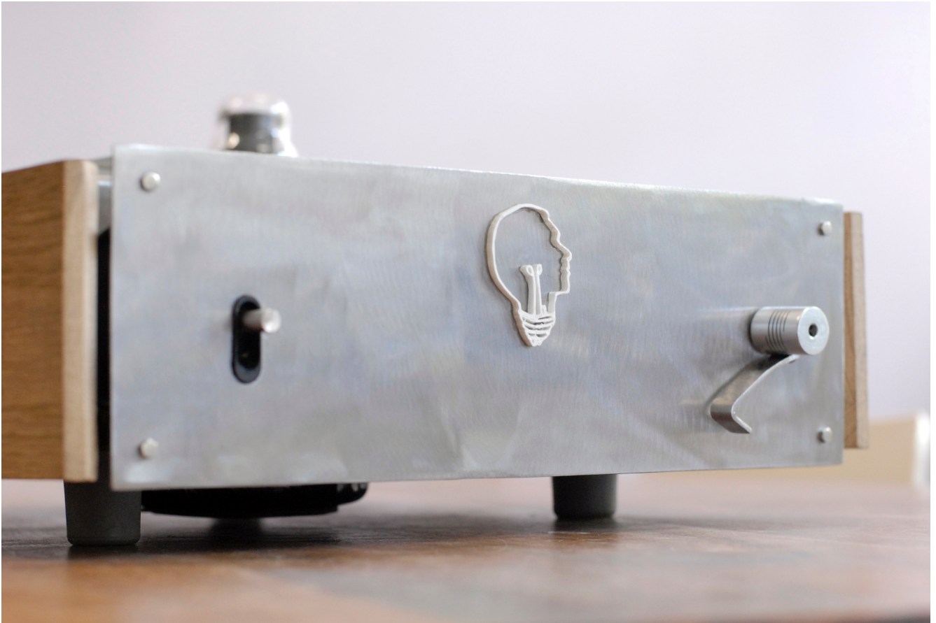
The front panel with the power switch of a Pioneer TX-5300. 3D printed logo and volume control. You can just see the power transformer hanging under the amplifier.
