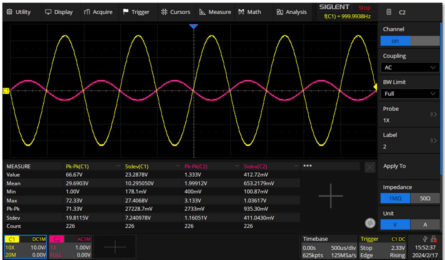
Figure 44 - Voltage levels just before clipping starts
