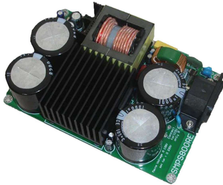
Figure 16 - Connex Electronics SMPS800RE Switched-mode Power Supply
