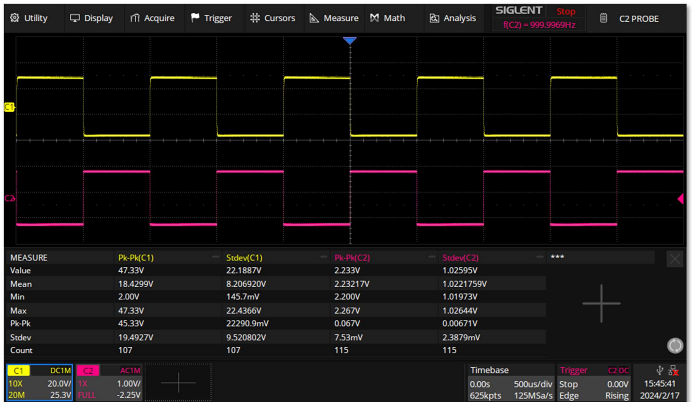
Figure 45 - Measurement of the output voltage (yellow) with a square wave at the input (red)
