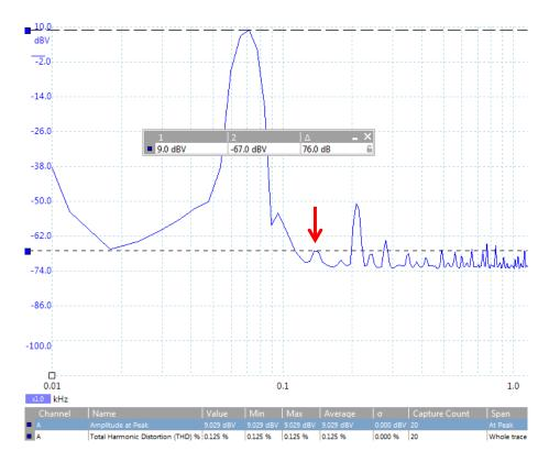
Fig. 6: AB test with 70 Hz signal +9 dBV (= 1 W in 8  $\Omega$ ) P4 is adjusted to minimize the 2<sup>nd</sup> harmonic component. 2<sup>nd</sup> harmonic now is -76 dB = 0,016 %
