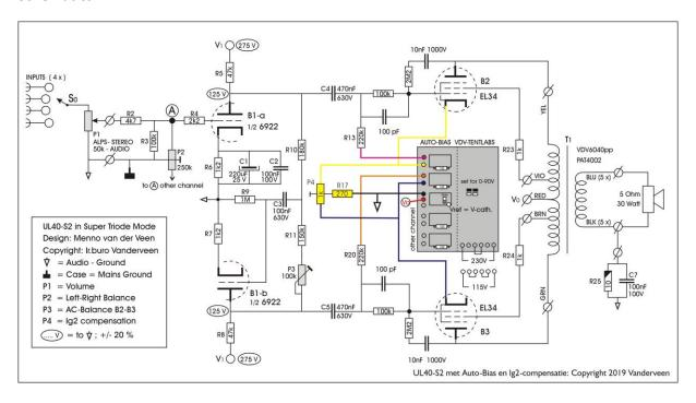
Fig. 1: UL40-S2 Auto-Bias circuit with  $I_{g2}$  compensation
