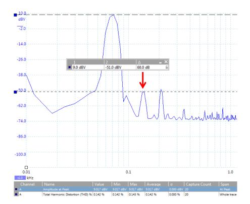
Fig. 5: AB test with 70 Hz test signal +9 dBV (= 1 W in 8  $\Omega$ ) With P4 in its mid position, no adjustment is made for differences in I<sub>g2</sub>.  $2^{nd} \text{ harmonic} = -60 \text{ dB} = 0,1 \%$
