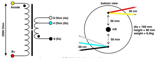
always connect all (5x) black lead outs together always connect all (9x) blue lead outs together always connect all (4x) white lead outs together
