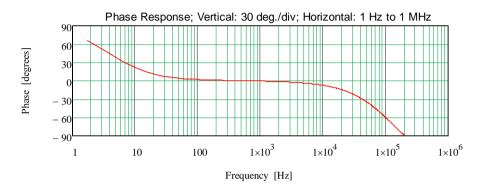
Differential Phase Response; vert. 30 deg./div; hor. 1 Hz to 1 MHz See: W.M.Leach, Differential Time Delay..; JAES sept.89 pp.709-715
